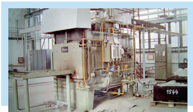
New technology in the new hardening shop - IPSEN hardening furnace
